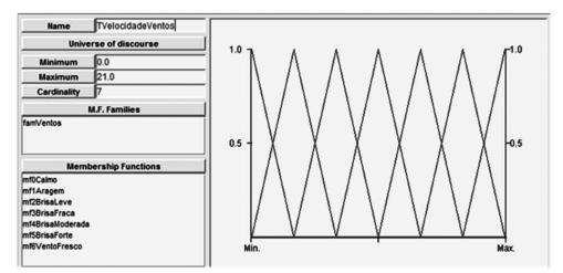
Figure 4 - A family of membership functions (BATURONE et al., 2007) for TVelocidadeVentos represented in XFUZZY based on the variables of the Beaufort scale (LISKA et al., 2013) Source: authors, (2015)
