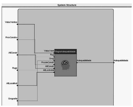
Figure 12 - Logical relationship between different types of variables fo wind profiling efficiency Source: authors, (2015)
