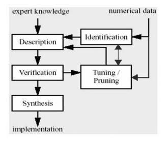
Figure 3 - Design methodology for Xfuzzy system Source: Barriga et al., 2007
