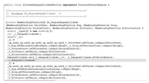
Figure 7 - part of the Java code created from XFUZZY from rule base graphical design above using xfj module
