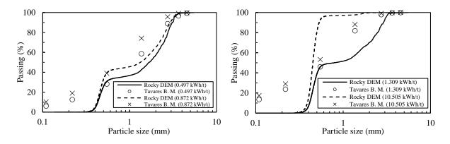
Figure 6 – Comparison between the modelled and simulated progeny size distributions for a single particle impact of particles of 5.47 mm for different impact energies for the limestone particles.
