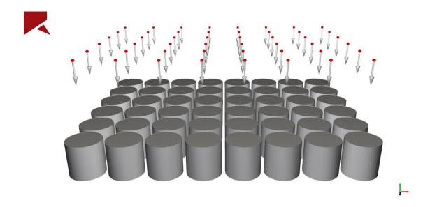
Figure 1 - Simulation setup of 48 single particle impact tests in DEM environment using particles of 5.47 mm.
