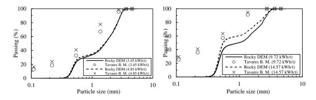
Figure 5 – Comparison between the modelled and simulated progeny size distributions for a single particle impact of particles of 5.47 mm for different impact energies for the copper ore particles.
