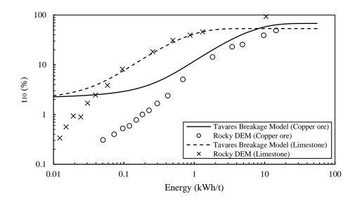
Figure 4 - Comparison between the modelled and simulated  $t_{10}$  values for a single particle impact of particles of 5.47 mm for different impact energies.
