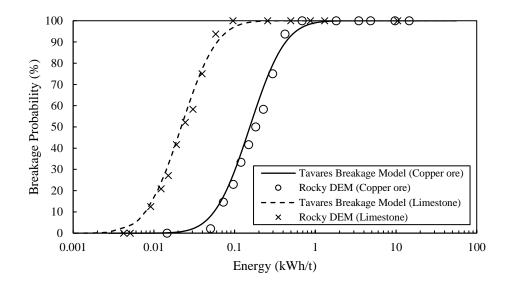
Figure 3 - Comparison between the modelled and simulated breakage probability for a single particle impact of particles of 5.47 mm for different impact energies.
