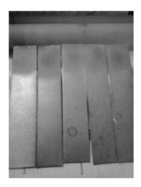
Figure 1: Specimens according to ASTM D 1002 (2010).
