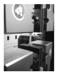
Figure 6: Adhesion tensile test (ASTM 638D, 2002).
