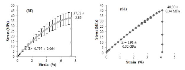
Figure7: Tensile test of the rapid curing and of the slow curing epoxy adhesive
