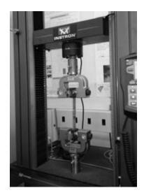
Figure2: Tensile Testing of single shear joints
