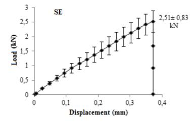
Figure 5: Lap-shear test of slow cure (SE) epoxy resin.
