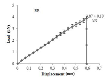
Figure 4: lap-shear test of rapid curing ((RE) epoxy resin.
