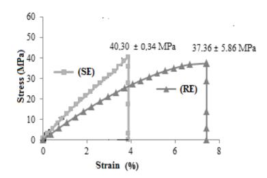
Figure 8: Comparison between rapid curing (RE) and of the slow curing (SE) epoxy adhesive (tensile test).
