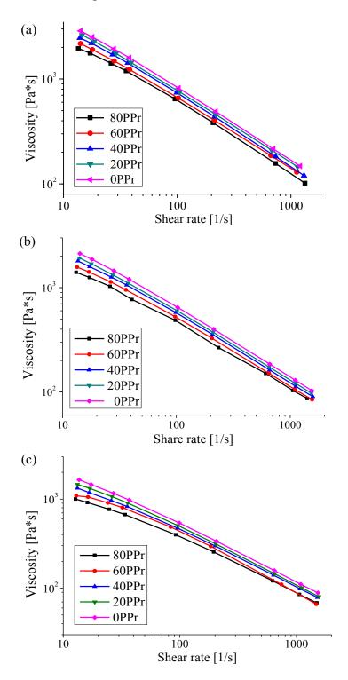
Figure 2- Viscosity of PPr/PPv blends with increasing shear rate at (a) 180°C, (b) 210°C and (c) 240°C.
