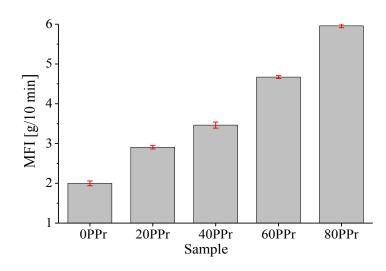
Figure 1- Variation of melt flow index of PPv and PPv/PPr blends.
