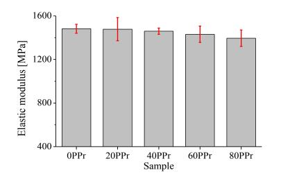
Figure 3- Elastic modulus of PPr/PPv blends.
